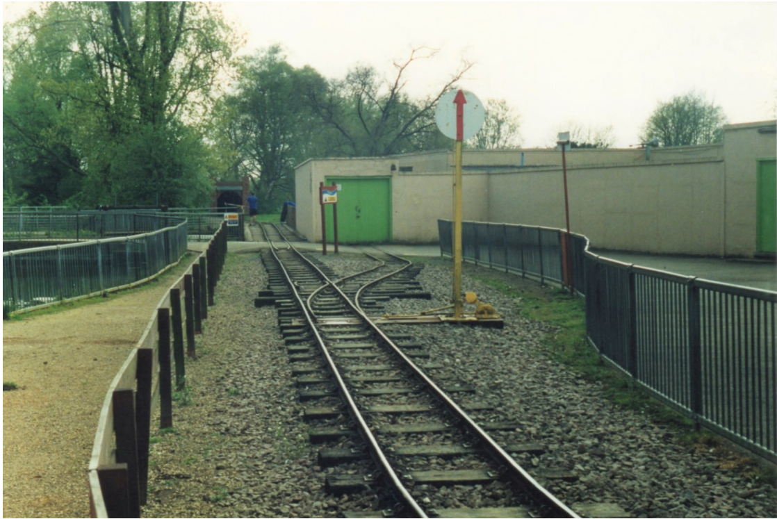
A view looking along the railway towards the siding leading into the engine shed. The tunnel can just be seen among the trees. The point indicator formed of a disc with an arrow can be clearly seen. The water chute is immediately on the left.
