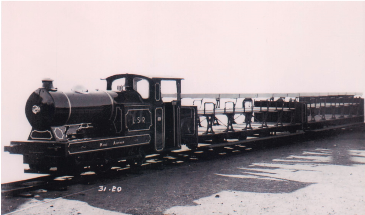
A Baguley works photograph of 2043 "King Arthur", with the two coaches that were completed by Baguley's. The locomotive is fully lined and painted – compare to photograph on page 20 where it is finished in works grey livery. (Baguley [Engineers] Limited. 1931. Reproduced by courtesy of Baguley Engineers Ltd, from original photograph held by Lichfield Record Office. Ref: B4288/C/2/302)
