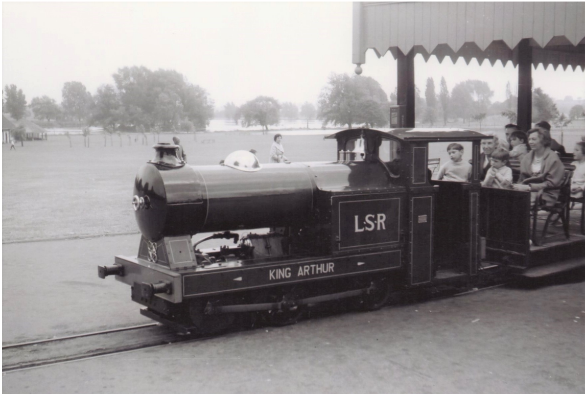
"King Arthur" waits to depart with some expectant passengers. The locomotive looks smart and well cared for. A cow-catcher and air brakes are yet to be fitted. (Sydney A Leleux. 6/7/62)
