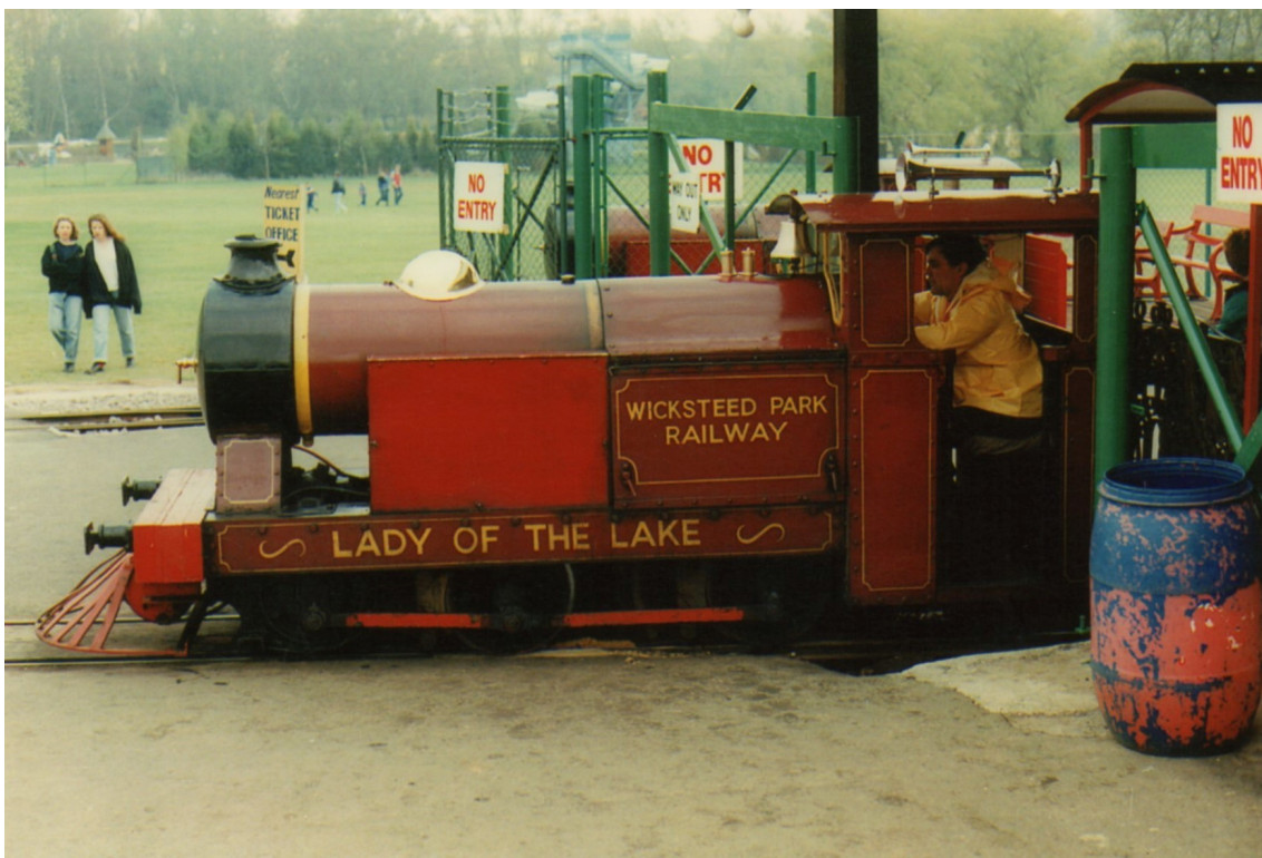
"Lady of the Lake" shows the modifications that came with air braking. Note the reservoir under the extended front buffer beam and extended side box. The locomotive has yet to be repainted to suit. "King Arthur" is just visible behind. (G Fairweather. c1991)
