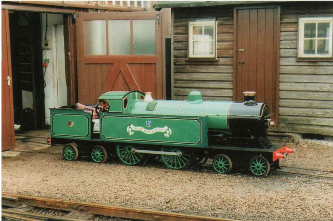
The first ever steam outline internal combustion locomotive, "Blacolvesley" built in 1909, employed a Wicksteed gearbox. This had been developed for the motor car industry but was a failure. Here we see the attractive 15" gauge 4-4-4T locomotive at Ravenglass. (D Holroyde. 26/4/97)
