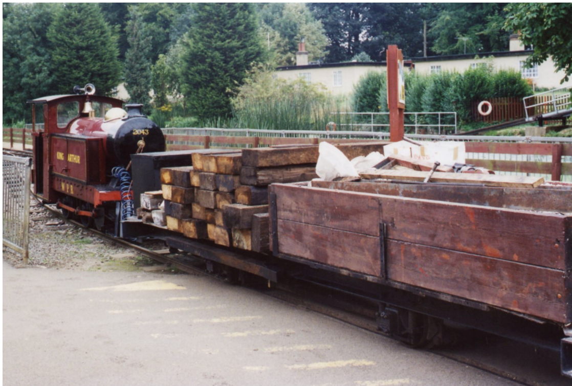
"King Arthur" has just pulled the maintenance wagon out of the engine shed (its normal stabling place). The wagon is built on a former Baguley coach frame and is air braked.
