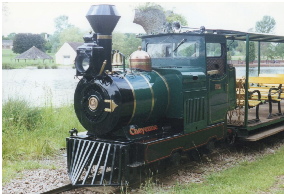
By way of a comparison, here is a view of "Cheyenne" by the siding leading into the workshop. This was the only steam outline locomotive built as such by Motor Rail Ltd, although other examples were converted later by their owners.
